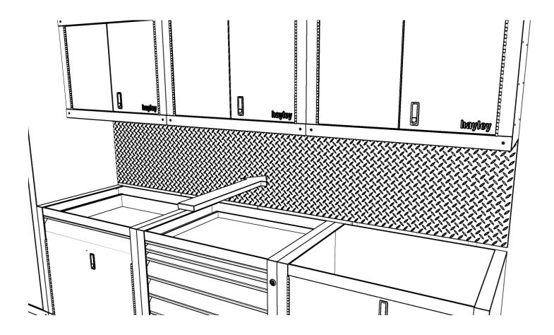
Add the counter top with the holes facing to the front. Line up the counter holes with the matching holes in the cabinet. Insert the round headed 3/4" bolts into the front counter.
