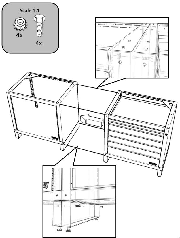
Once lower cabinets and closets are combined, level the unit in place. Make sure cabinet legs are adjusted to where they are touching the floor. This can be done by hand with final adjustments made with a wrench.
